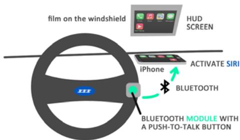
**Figure 2.** A used car without built-in IVIS
